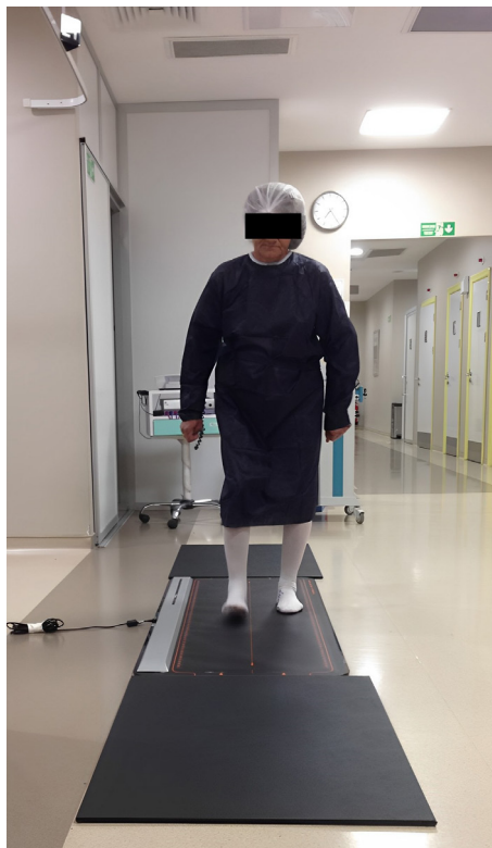
Fig. 2. Analysis of the spatiotemporal gait parameters on Win-Track platform.
